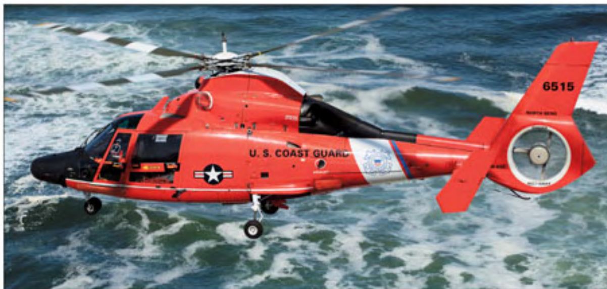
Right and upper-right: The French Dauphin (Dolphin) was first acquired by the Coast Guard during the mid-eighties from what was then Aérospatiale Helicopter (later Eurocopter). Ninety-six HH-65As were delivered 'green' for outfitting at its subsidiary in Grand Prairie, Texas. The design incorporated several new technologies of the day, like a composite rotor head, fibreglass rotor blades and a shrouded, 11-blade tail rotor.
