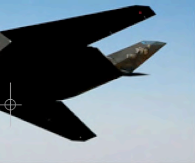
Above and left: For 25 years the F-117 has been blazing the trail of stealth operations. Despite its aerodynamics being seriously compromised by the over-aggressive need to reduce radar cross-section, the aircraft is quite manoeuvrable and can be flown quite aggressively by an experienced pilot. The F-38 companion trainer is nimble enough to keep up with the Nighthawk throughout training sorties.
