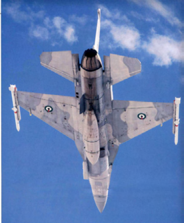
The second F-16F has two forward-facing, gimballed Schneider Kreuznach Cinecam C-mount high-speed video cameras mounted just inboard of the tailplanes to record weapon separations. Three further cameras are carried in each AIM-120C AMRAAM digital camera pods on the wingspans, facing inwards.
