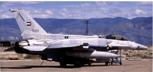
The second F-16F has two forward-facing, gimballed Schneider Kreuznach Cinecam C-mount high-speed video cameras mounted just inboard of the tailplanes to record weapon separations. Three further cameras are carried in each AIM-120C AMRAAM digital camera pods on the wingspans, facing inwards.
