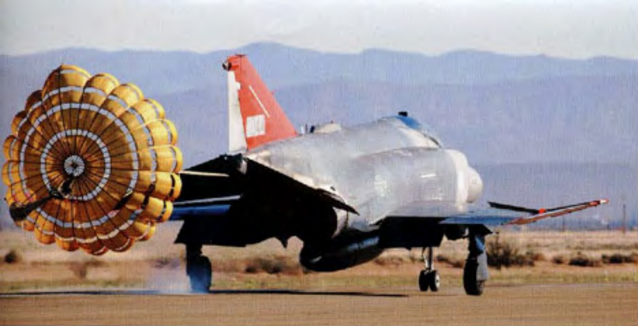
A QF-4 returns from a routine manned sortie. For unmanned operations the aircraft is stopped on the 'droneway' by an arrestor wire system. This, however, takes some time to reset before another drone can be recovered.
