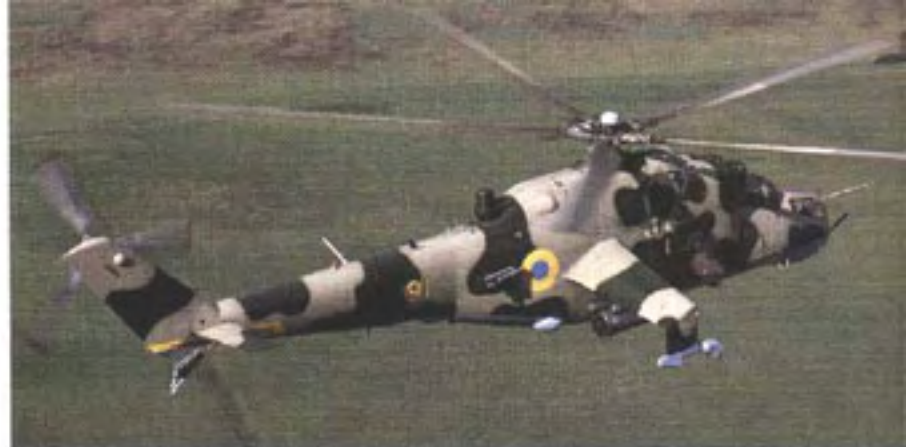
above: Among Ukraine's 'Hind' inventory are a small number of Mi-24Rs. The Mi-24R was developed specially for the NBC (nuclear, biological, chemical) reconnaissance role.
